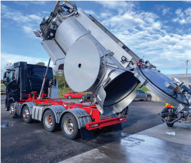
A recent addition is this four-axle Volvo truck with a 10,000-litre stainless-steel tank.
